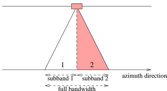
**Figure 1.** Illustration of the azimuth decomposition into 2 sub-bands.
