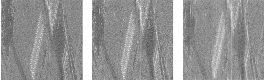
**Figure 2.** From left to right: original image, left sub-band and right sub-band obtained after a 2-sub-band azimuth decomposition.
