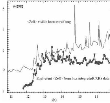
**FIGURE 1.** Comparison of the line averaged  $Z_{\text{eff}}$  from visible bremsstrahlung and its equivalent CX line integral reconstructed from contributions of  $\text{C}^{6+}$ ,  $\text{Be}^{4+}$  and  $\text{He}^{2+}$  on the JET tokamak.
