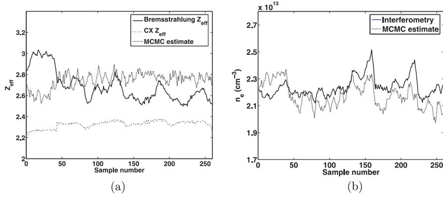
**FIGURE 2.** (a) Central line-averaged  $Z_{\text{eff}}$  determined from bremsstrahlung measurements in a series of TEXTOR discharges, central  $Z_{\text{eff}}$  from carbon density measurements by CXRS and the estimated  $Z_{\text{eff}}$ . (b) Central electron density from interferometry in a series of TEXTOR discharges, and its estimate by the MCMC sampling procedure.
