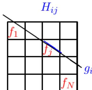
$$\begin{aligned} f(x, y) &= \sum_j f_j b_j(x, y) \\ b_j(x, y) &= \begin{cases} 1 & \text{if } (x, y) \in \text{pixel } j \\ 0 & \text{else} \end{cases} \end{aligned}$$
