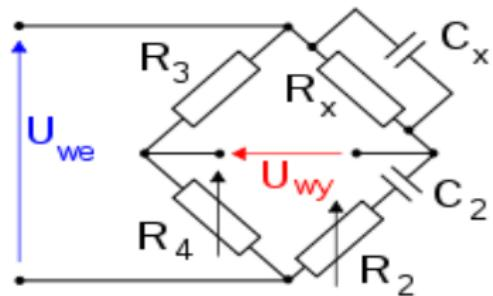
At some frequency, the reactance of the series R<sub>2</sub>C<sub>2</sub> arm will be an exact multiple of the shunt R<sub>x</sub>C<sub>x</sub> arm. If the two R<sub>3</sub> and R<sub>4</sub> arms are adjusted to the same ratio, then the bridge is balanced.
