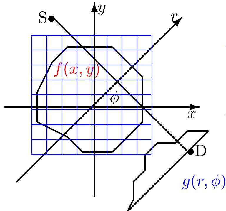
$$g(r, \phi) = -\ln \left( \frac{I}{I_0} \right) = \int_L f(x, y) \, dl$$
