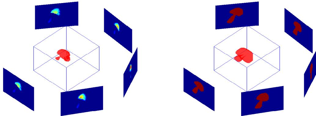
$$f(\vec{r}) = \begin{cases} 1 & \text{if } \vec{r} \in \mathcal{C} \\ 0 & \text{elsewhere} \end{cases} \quad g_i(x, y) = [\mathcal{H}_i f(\vec{r})](x, y) + \epsilon_i(x, y), \\ \mathbf{g}_i = \mathbf{H}_i \mathbf{f} + \epsilon_i = \mathbf{H}_i(\mathcal{C}) + \epsilon_i, \quad i = 1, \dots, M$$
